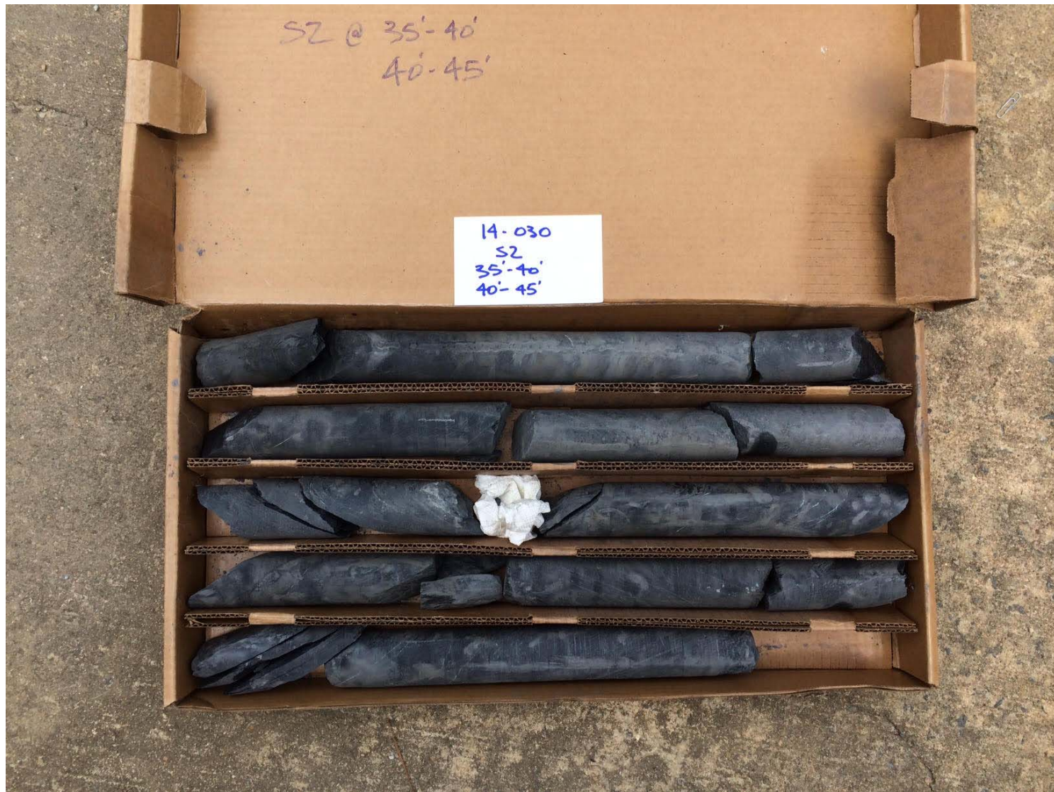
Rock Core - Boring S2 (Sta 1128+55, 110' Rt), 35 to 45 ft AHTD JOB CA0608 I-630 over Rodney Parham Road
