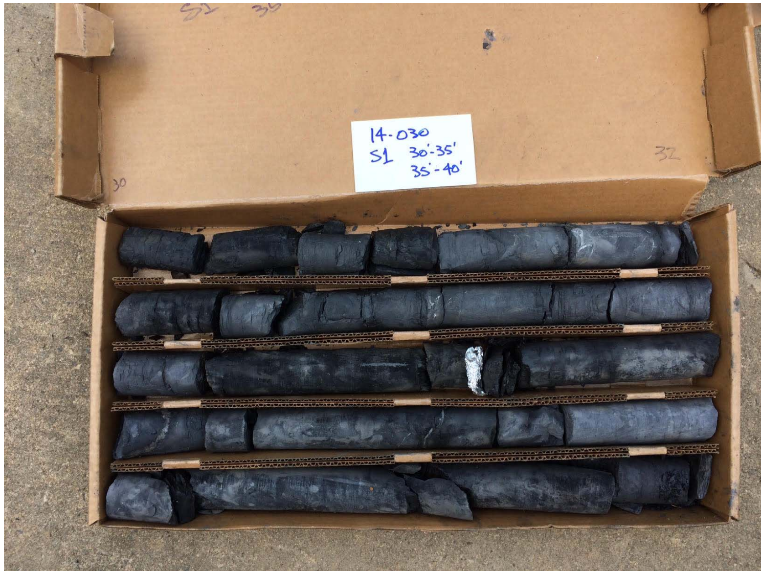
Rock Core - Boring S1 (Sta 1127+10, 70' Rt), 30 to 40 ft AHTD JOB CA0608 I-630 over Rodney Parham Road
